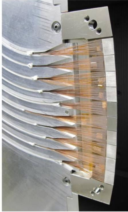
Figure 4: The pseudo-slit within the instrument that lines up the ten v-groove blocks, each containing 30 fibers, that are connected to the MTP connectors at the gang connector system.
