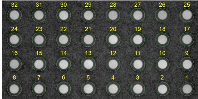
Figure 11: Fiber tips of a polished MTP as imaged by the DORC interferometer as part of an automated check of surface topography.
