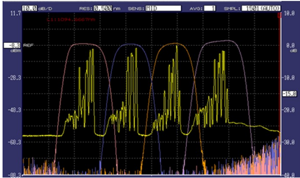
Figure 16a. Overlay of VCSEL and filter spectra.
